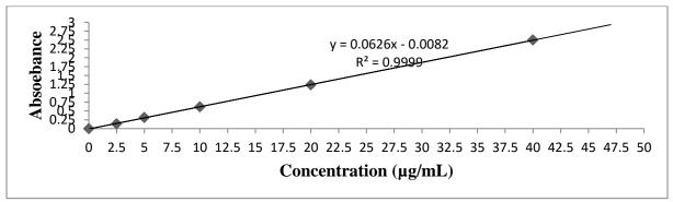
Figure 4: Calibration curve of levofloxacin-bromothymol complex for spectrophotometric assay
